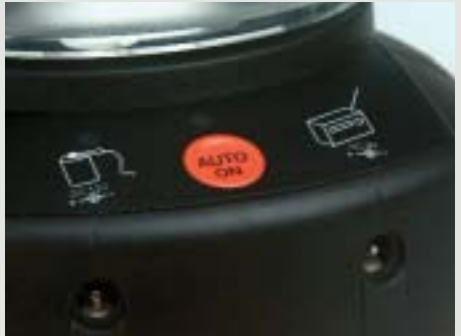
DC input from 12V solar module, mains adaptor or vehicle cigarette-lighter socket
