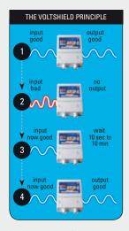
Surge and spike protection is also incorporated to ensure protection against these events which are very common. Surges and spikes are generated by lightning and nearby switching off and on of other equipment such as lighting, pumps, motors, compressors, elevators etc.
