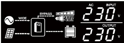
Even if AC input is absent, PV power can still charge the battery and the display will be as shown below.
