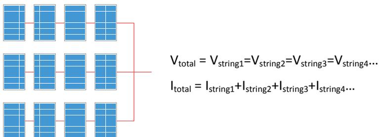
In either case, the total output power is  $P_{total} = P_{panel} \times \text{Number of PV panel}$
