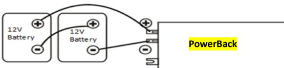
The user may connect the batteries in parallel in order to increase the total battery capacity without changing the battery voltage. The example below shows parallel connection of multiple 12V batteries. While the total capacity is times by the number of battery, the terminal voltage remains 12V.
