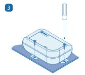
Using a screwdriver, tighten the two screws to secure the GMC5 to the surface.
