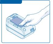
Remove the lining from one side of the pad and stick on the base of the GMC4
