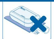
Ensure there are no pipes or wires behind the panel where the GMC4 is to be mounted.
