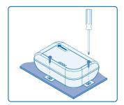
Using a screwdriver, tighten the two screws to secure the GMC4 to the surface.
