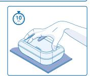
Remove the lining from the pad and immediately press the GMC4 into position.
