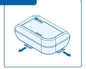
Pull out the screw mounting tabs from the bottom of the GMC4.
