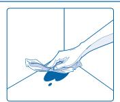
Clean contaminates from the installation surface with the alcohol wipe and dry.
