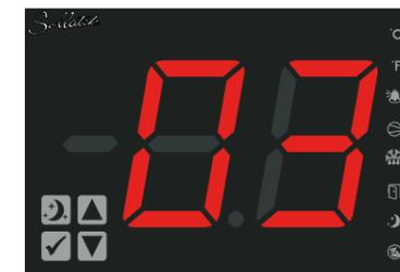
The measured temperature can be adjusted to display an off-set temperature
