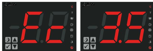
To manually force the controller in/out of Eco mode, press and the display will beep to and then will enter/exit eco mode.
