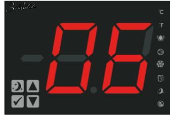
FTB - The differential temperature from the Eco set-point to turn the compressor ON.
