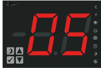
The temperature to turn the compressor OFF in ECO mode.
