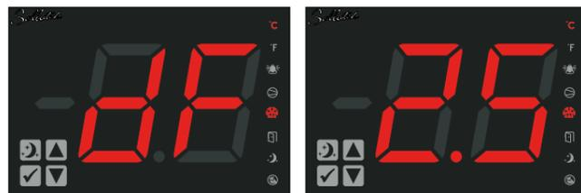
To manually force the controller in defrost mode, press & hold together until the display beeps (about 5 seconds).
