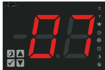
The duration between the finish of a defrost cycle and the start of the next one, if not started due to temperature.
