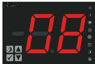
The duration of a defrost cycle if not ended due to temperature.
