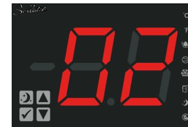
FTB - The differential temperature from the set-point to turn the compressor ON.
