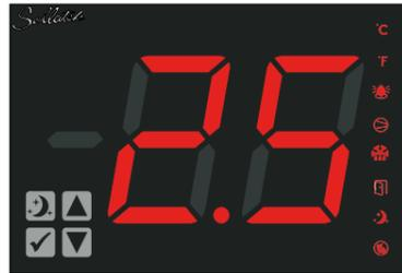
The live temperature and controller mode/statuses are shown on this screen as well as any alarms.
