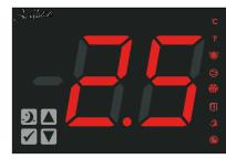
The live temperature and controller mode/statuses are shown on this screen as well as any alarms.
