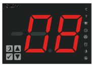
The duration of a defrost cycle if not ended due to temperature.
