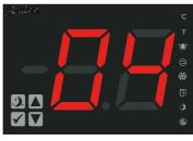
The duration for the door to stay closed to start Energy saving mode
