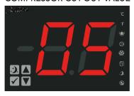
The temperature to turn the compressor OFF in ECO mode.
