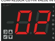
FTB - The differential temperature from the set-point to turn the compressor ON. FDEx2 - The temperature value to turn the compressor ON.
