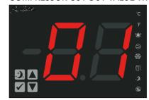
The temperature to turn the compressor OFF.
