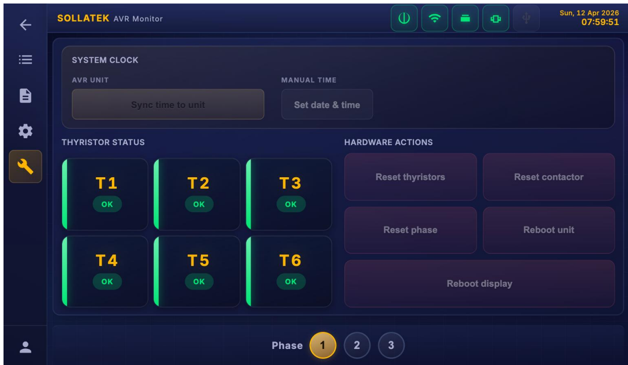
Fig 12: Settings > Maintenance with thyristor status grid and hardware action buttons
