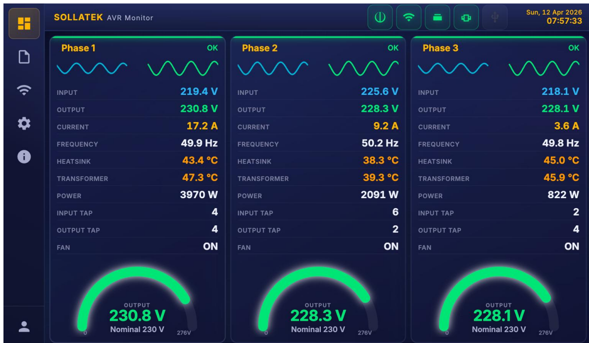
Fig 1: Overall layout showing side bar, top bar, and content area (Dashboard visible)
