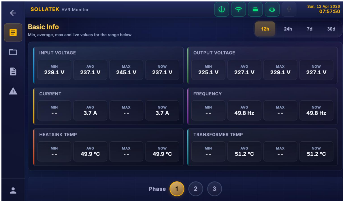
Fig 2: Logs > Basic Info view with statistics grid, time range pills, and phase selector
