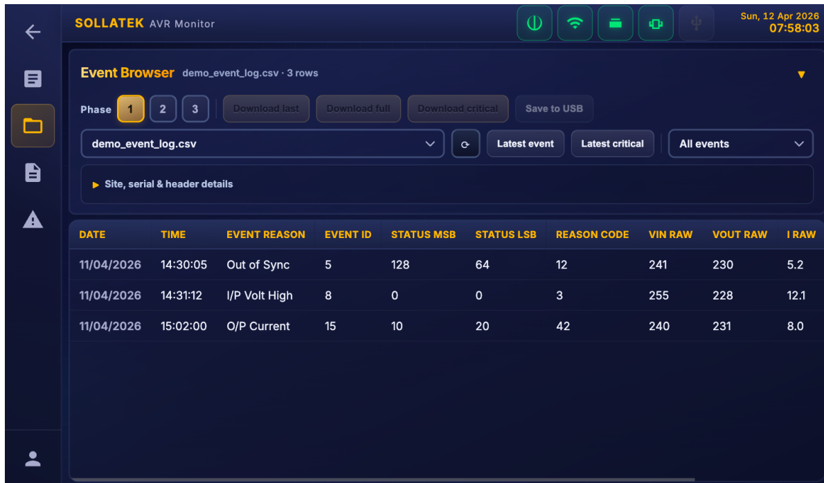
Fig 3: Logs > Event Browser with toolbar, file selector, filter, metadata, and CSV table
