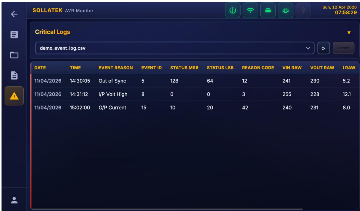
Fig 5: Logs > Critical Logs sub-view with file selector and CSV table
