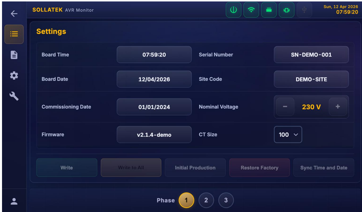
Fig 9: Settings > Basic with configuration fields, stepper controls, and action buttons
