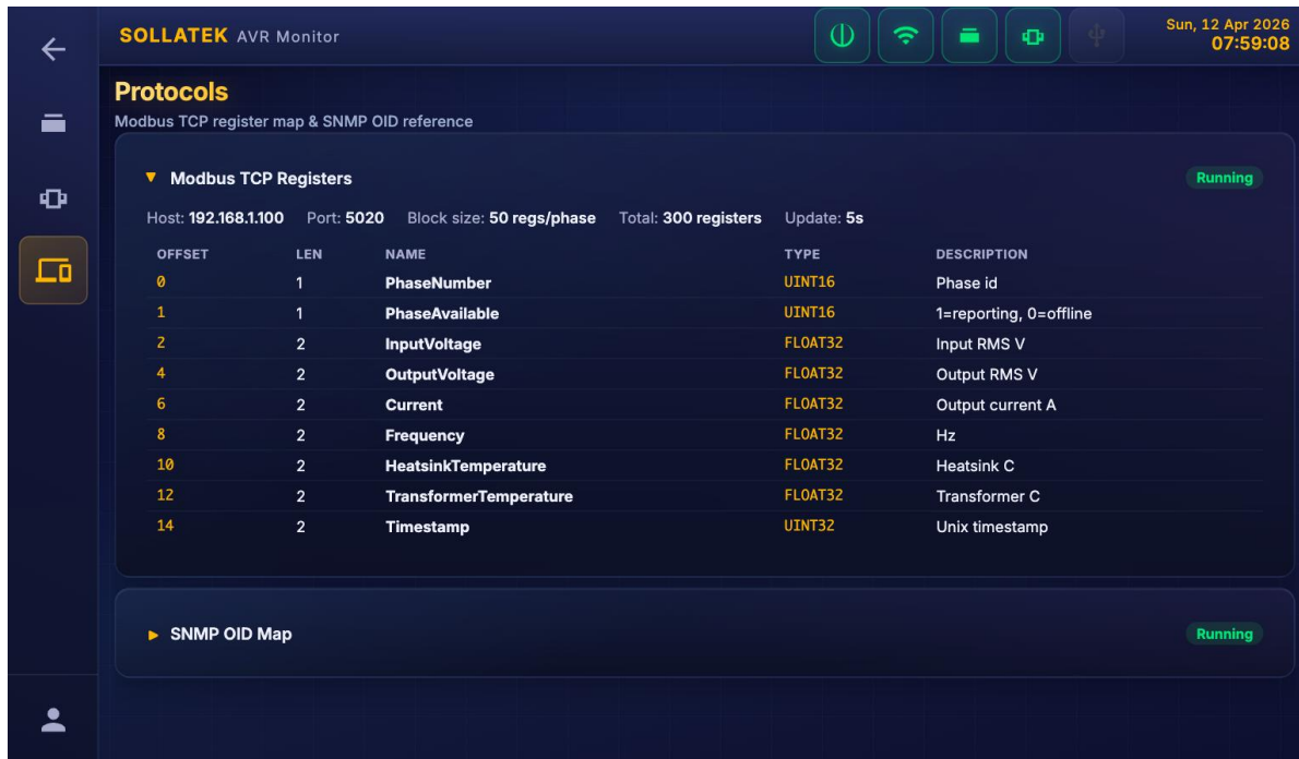
Fig 8: Connectivity > Protocols view with Modbus register map and SNMP OID reference
